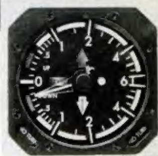
MODIFIED vertical speed indicator, CAS cockpit display by McDonnell Douglas, orders one plane (above) to climb; other, to dive. Each pilot limits the rate of climb or descent so that the pointer does not reach lighted area
